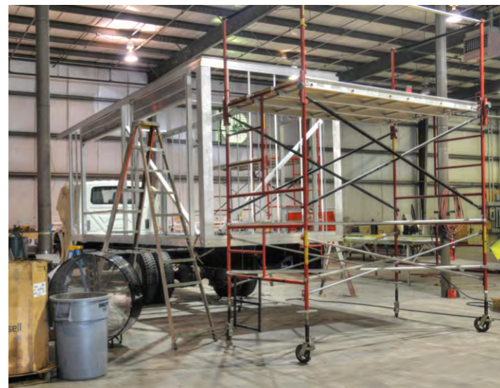
(right) A new mobile unit body under construction at LifeLine's 100,000 sq. ft. production facility in Columbus, Ohio
